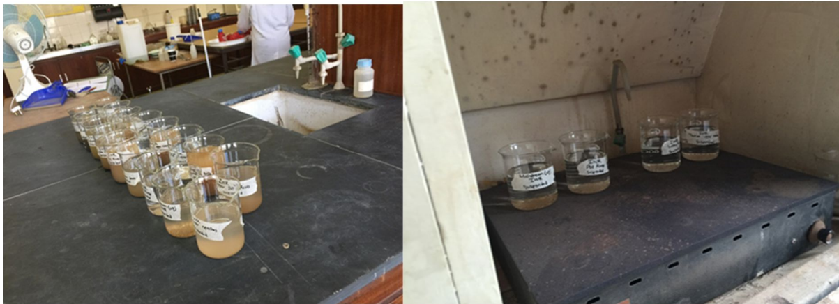
Figure 2. 10: Sediment samples left to settle out of solution (left photo) and evaporated samples(rightphoto).
