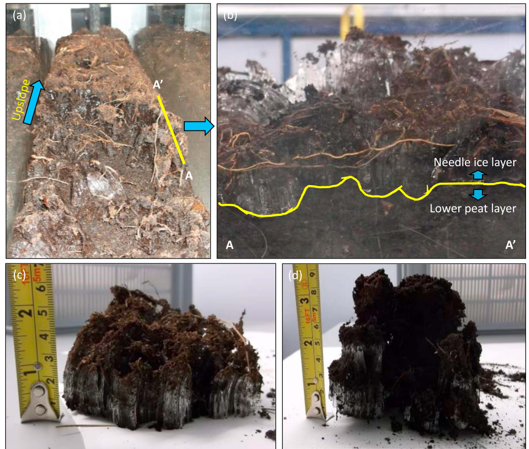
Figure 2. Morphology of laboratory needle ice growth: (a) Peat block with needle ice formation within the upper peat layers; (b) view from A-A' cross section of the peat block. Two distinctive layers including the upper needle ice layer and the much denser undisturbed peat layer below were identified; (c and d) typical needle ice formations. Note the friable surface layer resulting from formation of needle ice on the upper surface of the ice mass.
