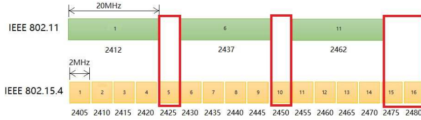
Fig. 1. The Channel Distribution of IEEE 802.15.4 and IEEE 802.11
