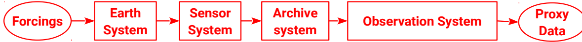
Figure 1: General overview of the various processes that lead to the proxy palaeodata used in climate reconstructions. In the example of pollen, the sensor system is the plant eco-system. The archive systems are the lakes or mires where pollen is deposited. The observation system includes the field and laboratory measures such as core sampling, pollen counting, and radiocarbon dating amongst others.
