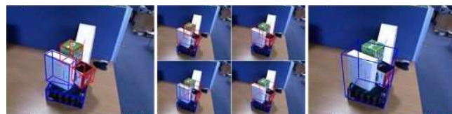
Figure 15: Output of Jia et al. [2013] on a scene with severe occlusion. Stable cuboids are shown in blue and unstable ones are shown in red. Given the ground truth segmentation, initial boxes are fitted after adjusting their orientation based on the supporting relations (left). In order to reach the physical stability, the algorithm merges neighboring segments during the optimization (middle). The optimized result is to merge all the regions to be stable (right).
