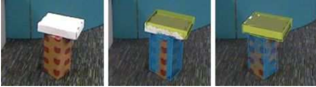
Figure 6: The initial cuboids (middle) are adjusted to better align the original image edges in the RGBD data (left) to produce refined cuboid candidates (right).
