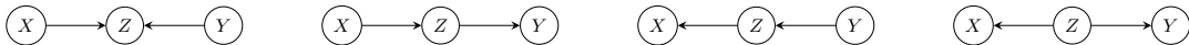
Figure 2: While in the left causal structure X \perp\!\!\!\perp Y , the other three networks share the conditional independence relation X \perp\!\!\!\perp Y | Z . This illustrates that the conditional independences are not sufficient to characterise the causal links among a set of random variables.
