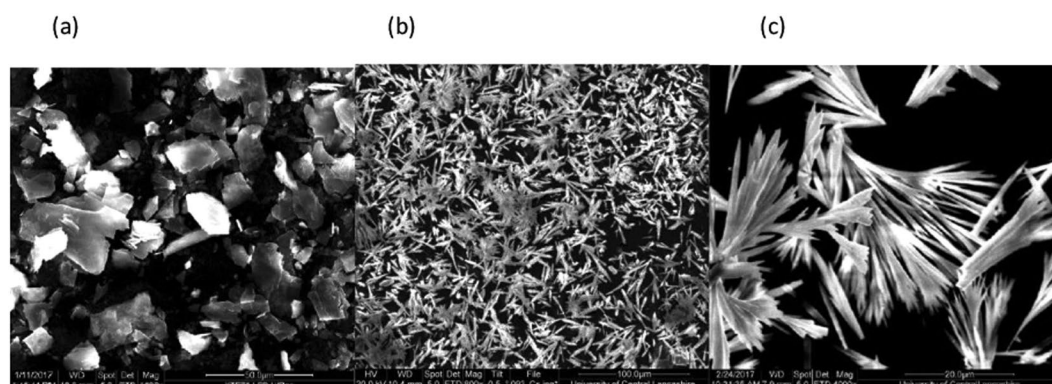
Figure 1. SEM images of FeAP platelets, ZnAP flowers and SnHP rods.
