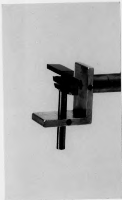
Photo 5.3. A four-reflection beam conditioner with a strain-relief cut for mounting.
