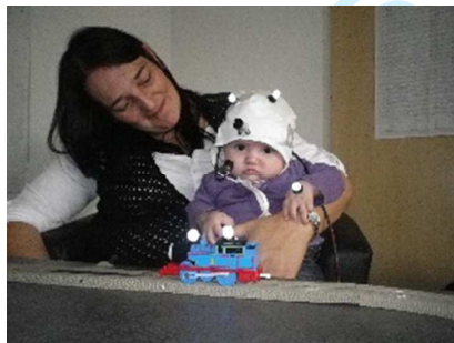
Figure 7 Infant wearing head set with eye tracker and field camera with motor markers mounted on the hands and the moving object. A binocular eye tracker could measure eye movements, while a field camera measured the entire spatial field in front of the infant (Smith, Yu, & Pereira, 2011). Because the eye tracker is not positioned in front of the infants, there would be no interference with their hand movements. Infants at this young age tolerate the headset without trying to remove it. Note the motor tracker markers on the head, the hands and on the moving train. The mother is holding the infant on the left side.
