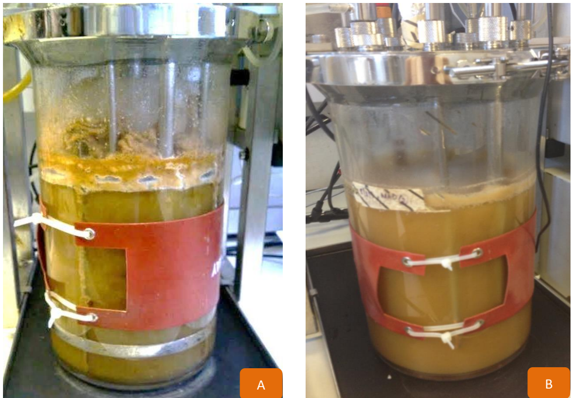
Figure 3.23: Fermentation of A. terreus in 5L Stirred tank reactor. a) Overgrowth of A. terreus in the headspace and the surface walls of the 5L bioreactor, b) A. terreus growth after bioreactor adjustments.
