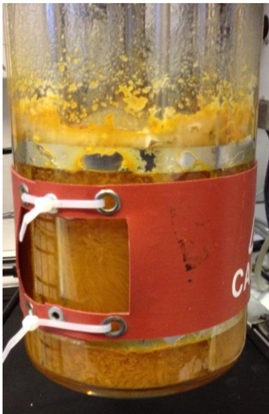
Figure 3.14: P. sclerotiorum fermentation in 2L STR. The orange colour represents P. sclerotiorum mycelial pellets.
