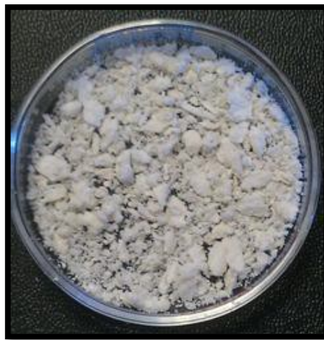
Figure 4.6: Freeze dried acetylated bacterial cellulose microcrystals used for composite production.
