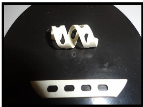
Figure 5.19: A stent prototype made up of P(3HO)/P(3HB) 50:50 blend film.
