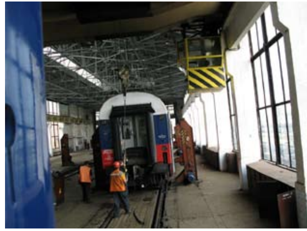
3.012 Preparing to lift the train carriages
