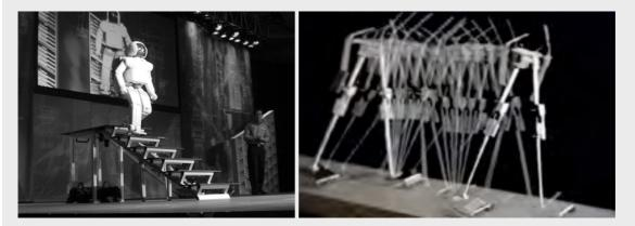
Fig. 5.4. Honda's Asimo (short for Advanced Step in Innovative Mobility). Asimo is a purely "top down" walking device, in that its movements are entirely driven by instructions to move motors, etc. It mimics the movements of a human, but uses lots of energy and computing power to do so (and is extremely expensive to make).
