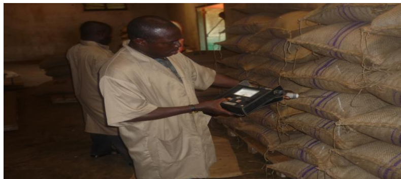
Figure 5.4 A QCD Officer using an Aqua-boy moisture meter to test the dryness of cocoa beans at a depot
