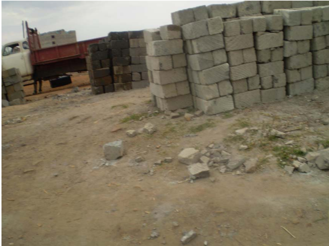
Plate 2: Machine-cut dimension stone at a stockist's yard in Kahawa, Nairobi.
