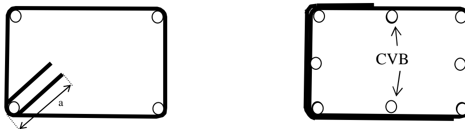
Figure 6.28: a) ACI 318 [6-5], Marti and Sarsam's proposed stirrup detailing at BCJ. b) This writer proposes detailing for external corner BCJ for torsion stirrups only when the structure is exposed to extreme loading which produce torsion at the joints.
