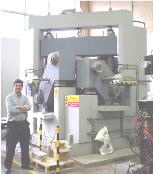
Figure 4.4: Triaxial stress testing machine at University of Sheffield, Department of Structural Engineering.
