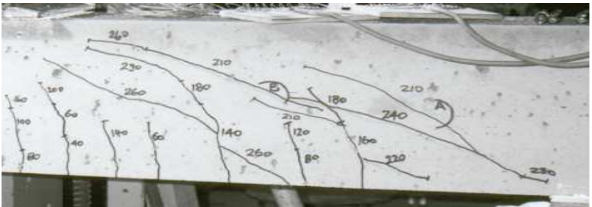
Figure 3.13: High Strength Beam (HSC2) with the angle of crack at about 43^\circ
