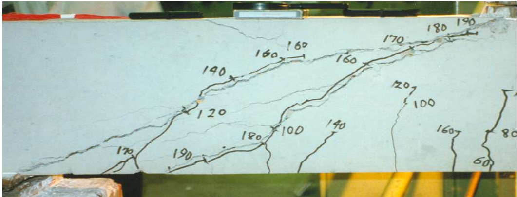
Figure 3.10: Normal Strength Beam (NSC3) with the angle of crack at about 27°
