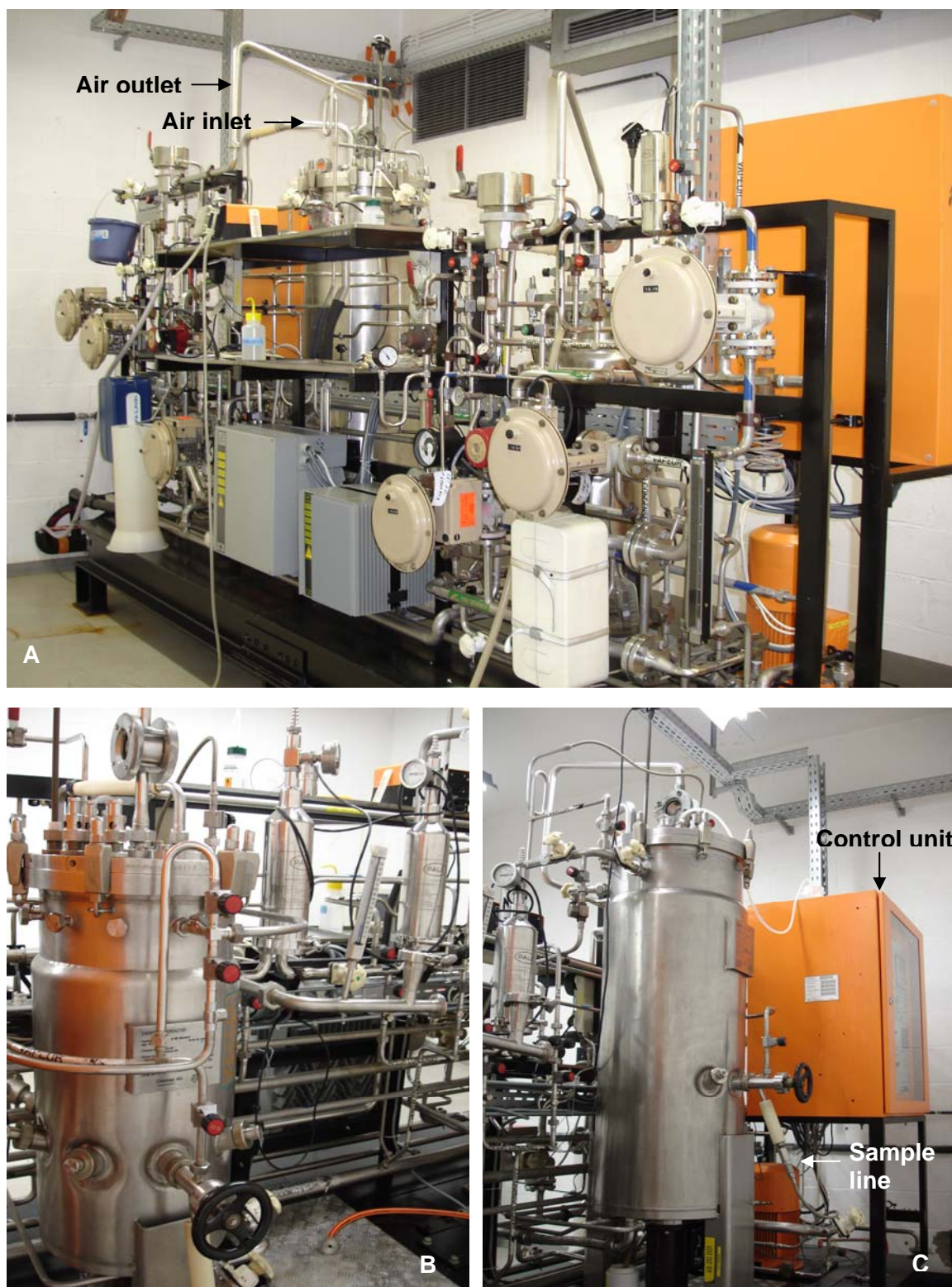
Figure 2.3: (A) The pilot scale fermenter system (Wetlands Engineering, Belgium) (B) 50 litre bioreactor (C) 150 litre bioreactor.
