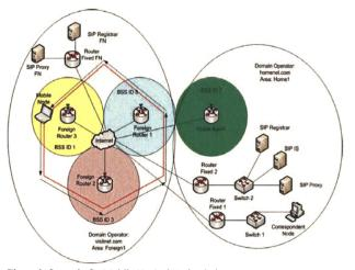
Figure 2. Scenario for Mobile IPv6 - SIP simulation
