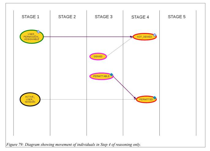
Figure 79 shows the movement of individuals in Step 4, in which PERMITTED is populated from PERMITTABLE and ACTIVE\_USER\_SESSION, and NOT\_DENIED from USER\_PERMISSION\_ASSIGNABLE and DENIED.
