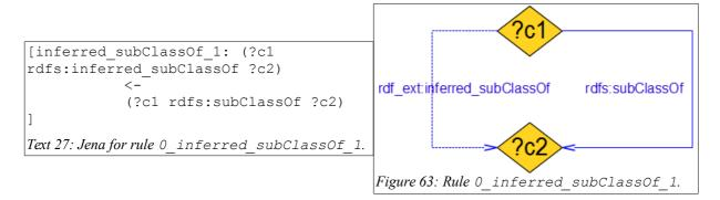
The first rule in Step 0, given in Figure 63, is called <code>0\_inferred\_subClassOf\_1</code>. It defines a class as being an inferred sub-class if it is a sub-class of that class. Figure 63 is converted into Jena syntax in Text 27 above.
