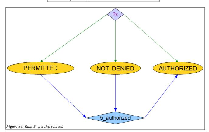
The second rule in Step 5, given in Figure 84, is called 5\_authorized. This defines AUTHORIZED as the intersection of PERMITTED and NOT\_DENIED: an individual is in AUTHORIZED if it is in both PERMITTED and NOT DENIED.
