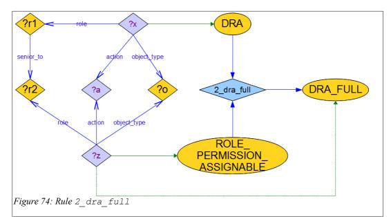
The first rule in Step 2, given in Figure 74, is called 2\_dra\_full. This rule moves an individual from ROLE\_PERMISSION\_ASSIGNABLE to DRA\_FULL if there exists an individual in DRA that has the same *action* and *object\_type* properties as that in ROLE\_PERMISSION\_ASSIGNABLE, and if the role property of the individual in DRA is senior to that of the individual in ROLE\_PERMISSION\_ASSIGNABLE.
