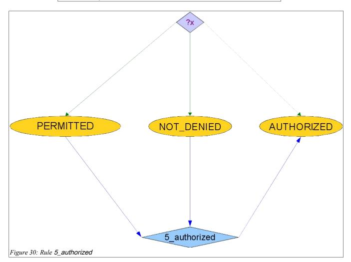
The second rule in Step 5, given in Figure 30, is called 5\_authorized. This defines AUTHORIZED as the intersection of PERMITTED and NOT\_DENIED: an individual is in AUTHORIZED if it is in both PERMITTED and NOT\_DENIED (Formula 6).
