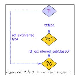
The fourth rule in Step 0, given in Figure 66, is called <code>0\_inferred\_type\_2</code>. It defines an individual as an inferred type of a class if it is a member of an inferred sub-class of this class. In other words, individual *?i* is an inferred type of class *?c* if it is a member of class *?c1*, which is an inferred sub-class of class *?c*.
