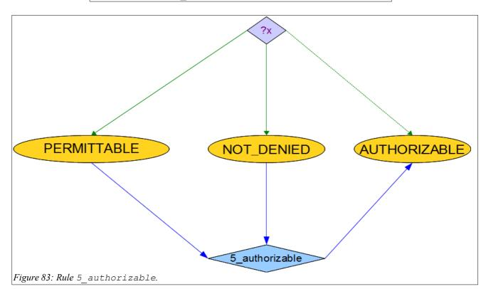
The first rule in Step 5, given in Figure 83, is called 5\_authorizable. AUTHORIZABLE is defined as the intersection of PERMITTABLE and NOT\_DENIED: an individual is in AUTHORIZABLE if it is in both PERMITTABLE and NOT\_DENIED (Formula 10).
