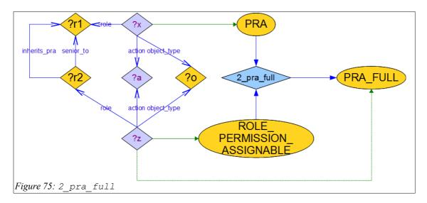
The second rule in Step 2, given in Figure 75, is called 2\_pra\_full. This rule moves an individual from ROLE\_PERMISSION\_ASSIGNABLE to PRA\_FULL if there exists an individual in PRA that has the same *action* and *object\_type* properties as that in ROLE\_PERMISSION\_ASSIGNABLE, and if the *role* property of the individual in PRA is junior to that of the individual in ROLE\_PERMISSION\_ASSIGNABLE.
