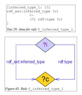
The third rule in Step 0, given in Figure 65, is called <code>0\_inferred\_type\_1</code>. It an individual as being an inferred type of a class if it is a type (member) of this class. Figure 65 is converted into Jena syntax in Text 29 above.
