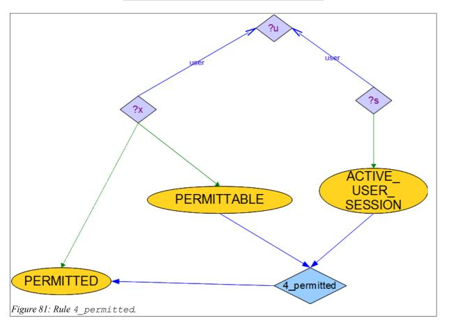
The second rule in Step 4, given in Figure 81, is called 4\_permitted. This rule moves an individual in PERMITTABLE to PERMITTED if the individual has a user that is also a user in an active user session, as given by an individual in the class ACTIVE\_USER\_SESSION. The difference between PERMITTABLE and PERMITTED is that PERMITTABLE represents potential permissions, while PERMITTED represents actual permissions, as determined by active user sessions.
