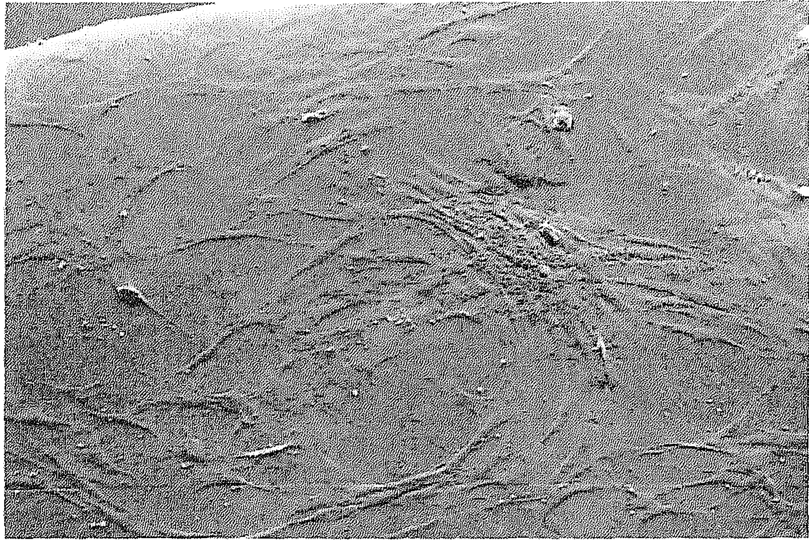
Figure 8. Scanning electron micrograph of RDF on an SilD00 surface after an incubation period of 3 days (1 division = 100 \mu\text{m} ). Note the random orientation.
