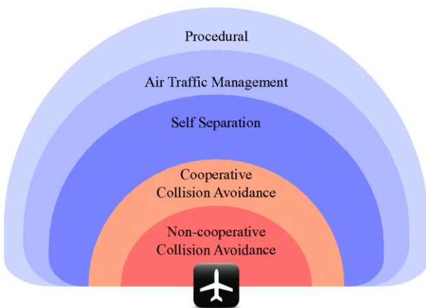
Figure 1. Separation and collision avoidance mechanisms.
