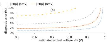
Fig. 12. Expected diagnosis error  $ER_x$  when a)  $V_{Vdd}@sb \le V_{dd}/2$ ; b)  $V_{Vdd}@sb > V_{dd}/2$
