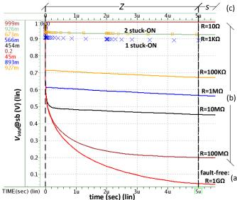
Fig. 9. AC analysis of bridges at power rails and stuck-on power switches
