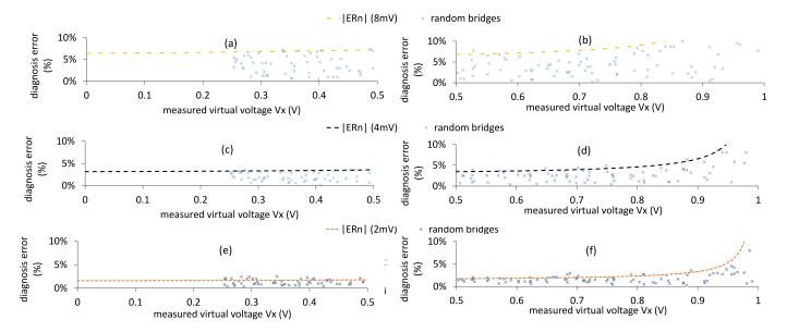
Fig. 14. Expected  $(ER_x)$  and actual ('x' points) diagnosis error for random bridges as a function of the measured virtual voltage  $(V_x)$  for sampling setups exhibiting a sampling error of (a)(b) 8mV; (c)(d)4mV; and (e)(f) 2mV; and bridges with (a)(c)(d)  $V_{Vdd}@sb < V_{dd}/2$ ; and (b)(d)(f)  $V_{Vdd}@sb > V_{dd}/2$
