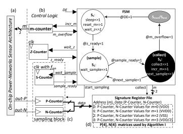
Fig. 10. Signature generation unit: (a) on-chip power-networks sensor; (b) signature generation control logic; (c) sampling block; (d) signature generation file and stored values of P. N-counters
