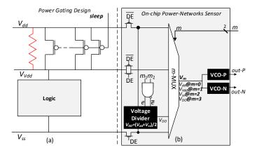
Fig. 7. The on-chip power-networks sensor architecture
