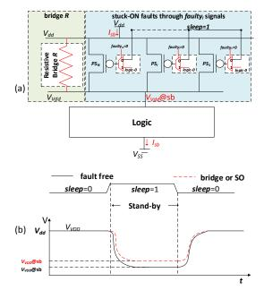
Fig. 1. (a) Power gating with header power switches and fault injection mechanism for resistive bridges and stuck-ONs; (b) impact of faults on the  $V_{Vdd}$  during the transition power-on $\rightarrow$ stand-by $\rightarrow$ power-on mode.
