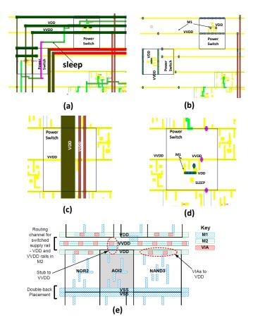
Fig. 2. Power rails and vias at the physical layout of power-gating design practices that can suffer by bridges: (a),(b) ring-style power gating; (c),(d) gridstyle power gating; (e) industrial practice of dRing power-gating. ((a)(b)(c)(d) are obtained from physical synthesis and (e) is reproduced from [16]).
