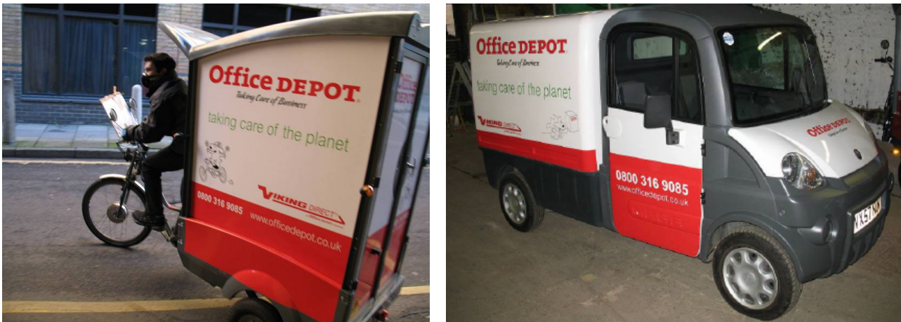
Figure 5: Cargocycle and electric van used in the City of London trial
