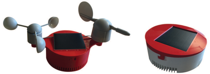
Fig. 2. The housings designed for the Master Node (on the left) and the Sub Node (on the right). Both nodes are equipped with a solar panel that sits on top of the housing to enable energy harvesting. As can be seen the master node has wind velocity and direction measurement instruments.
