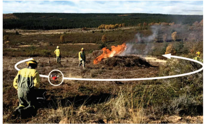
Fig. 5. The nodes are distributed in a circular fashion around the location of the fire. The white circle highlights one of the nodes
