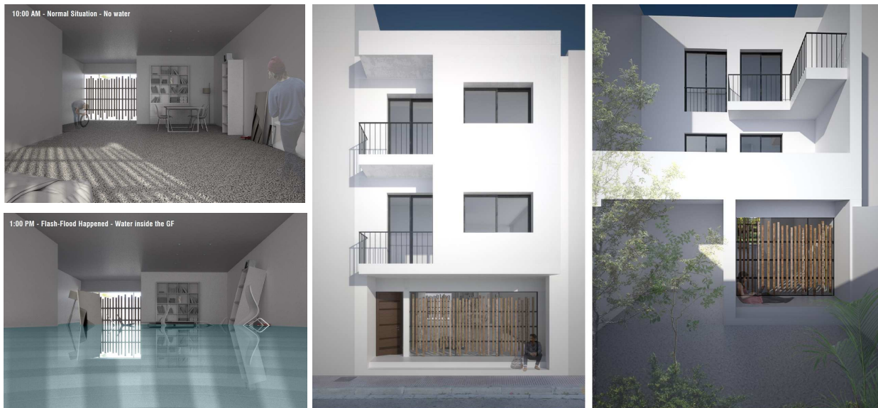
Figure 8. Virtual images of the of the proposed flood resilience design for Case Study 2: Terraced Apartment Building, with and without flood water, as it would be most of the time.
