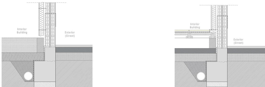
Figure 7. Two steps and a high suspended floor (right) and one step and gravel drainage floor (left) sections.
