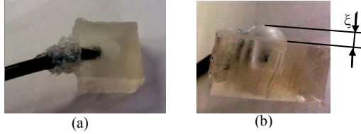
Figure 3. (a): Non-activated pneumatic haptic feedback actuator; (b): Activated pneumatic haptic feedback actuator.
