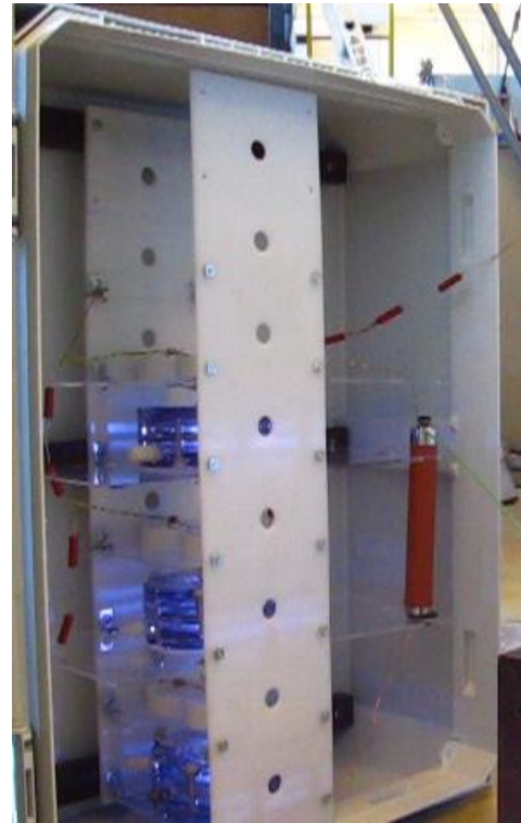
Figure 3. A photograph of the assembled generator, a transient discharge (light blue sparks) was captured.
