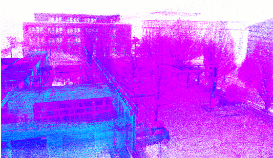
FIGURE 5.8: This figure shows intensity sensor data transformed with NOctoSLAM pose estimates from a combined indoor and outdoor episode. The sensor data was acquired by carrying the sensor through the DFKI Bremen building to the outside.
