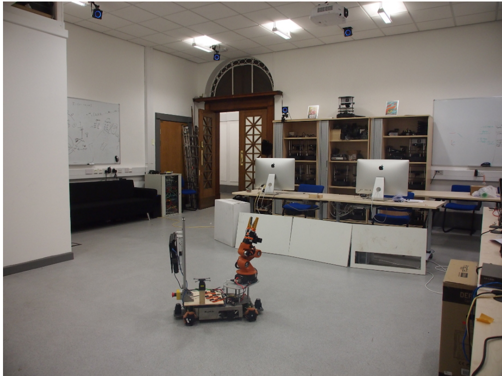
FIGURE 4.6: A photo of the environment the real robot experiments take place in, including motion capturing system and youBot.
