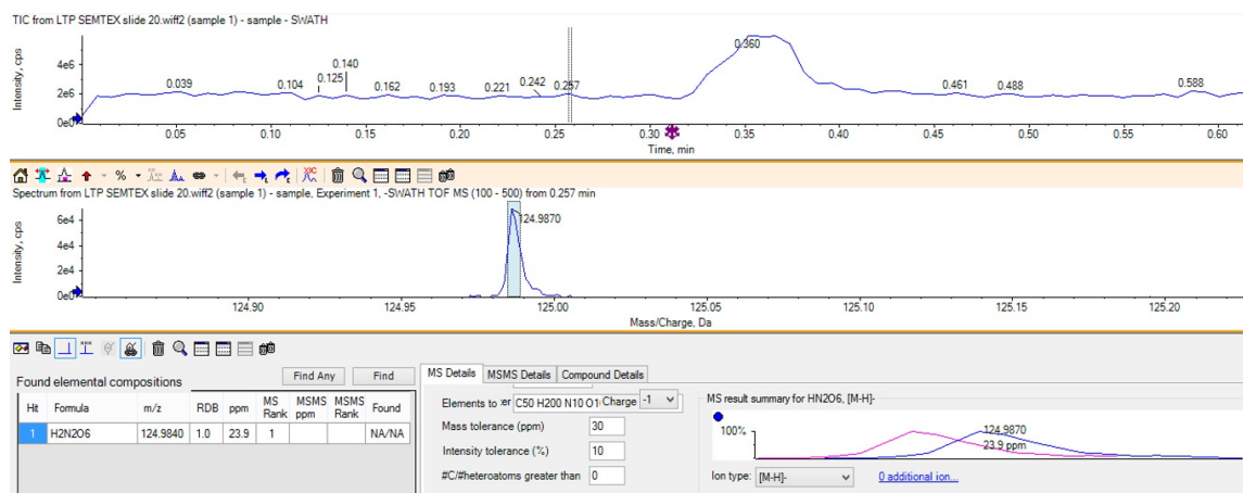
Figure 8.8. SWATH TOF/MS scan from a glass slide contaminated with Semtex where the sample is inserted between 0.30 and 0.40 min (top). Presented here (middle) is a background peak taken from ca. 0.25 min at m/z 124.9870 presumed to be [\text{HNO}_3(\text{NO}_3)]^- . Formula finder (bottom) identifies the peak to have the formula \text{H}_2\text{N}_2\text{O}_6 with a calibration shift of 23.9 ppm. Samples analysed via DBD coupled with a SCIex X500R QTOF.
