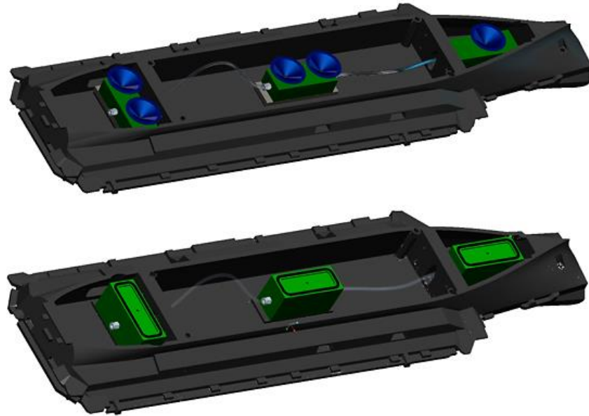
Fig 45: Competing QE-Class suction-block arrangements
