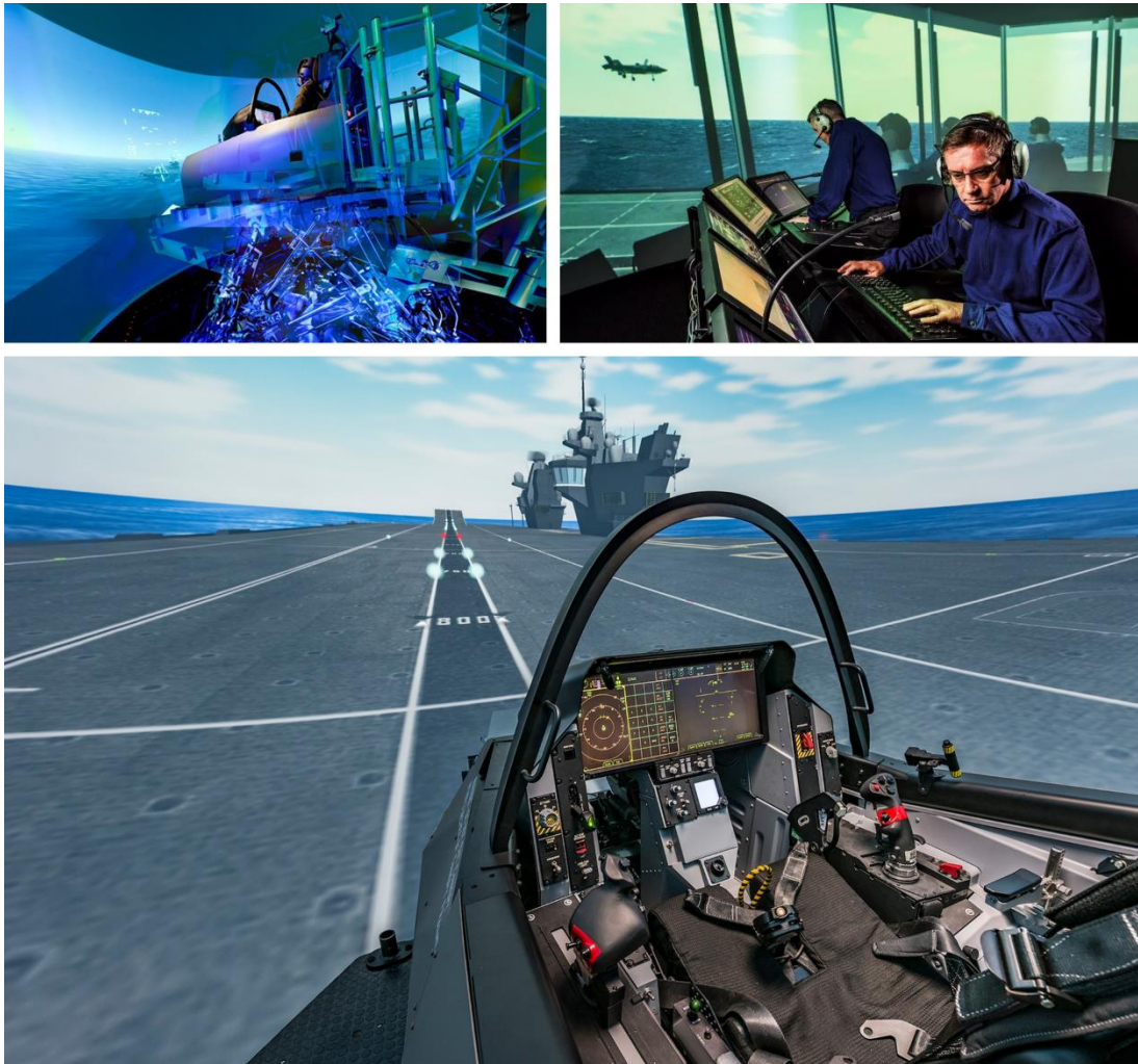
Fig 4: F-35B Simulation Facility at BAE Systems Warton, clockwise from top left: six degree-of-freedom motion base, LSO station, realistic F-35B cockpit and QEC visual environment (courtesy: BAE Systems)
