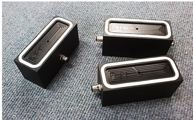
Fig 47: Prototype EPDM suction blocks
