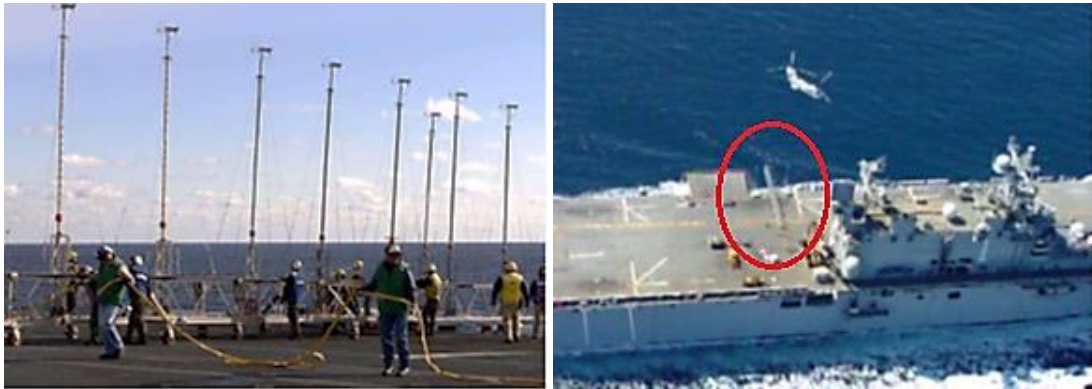
Fig 29: Anemometer rig aboard LHA-1 (Polsky, 2008)
