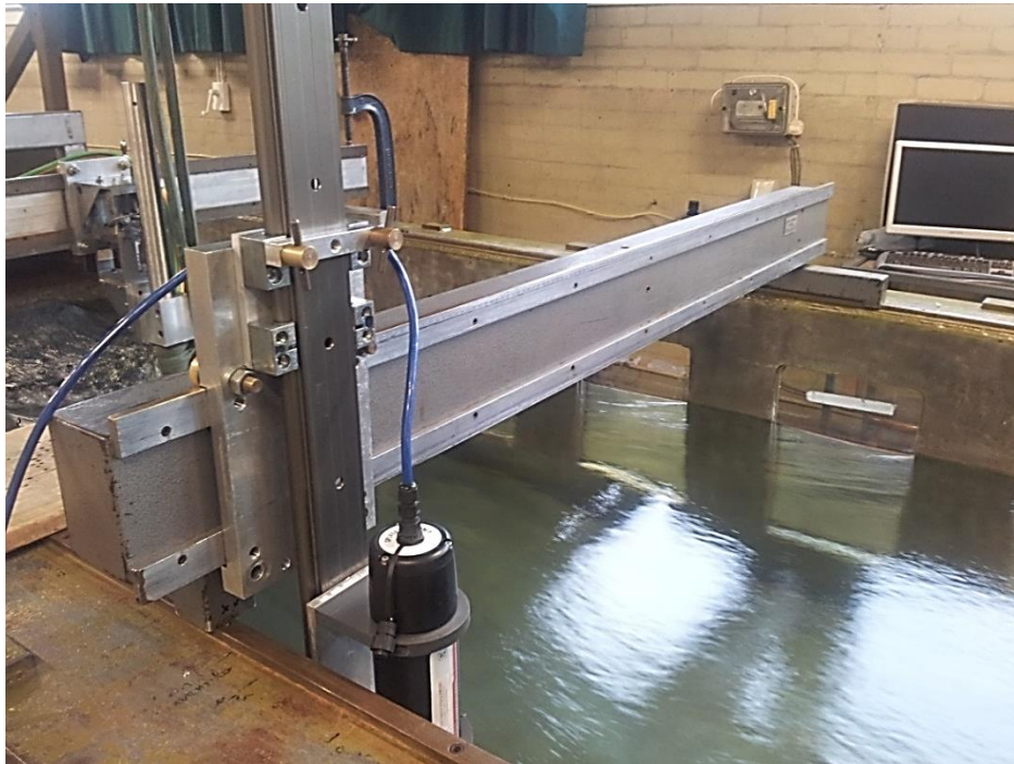
Fig 53: Pre-existing ADV traverse system
