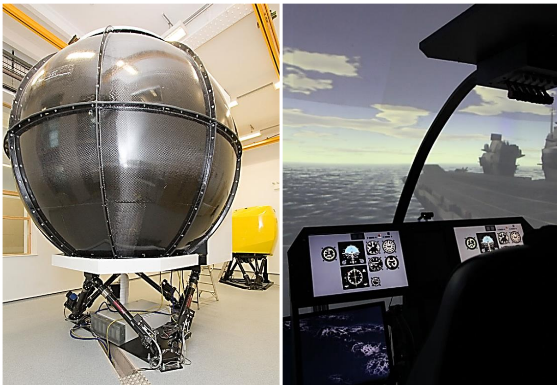
Fig 60: HELIFLIGHT-R piloted flight simulator (left foreground) with QEC visual environment
