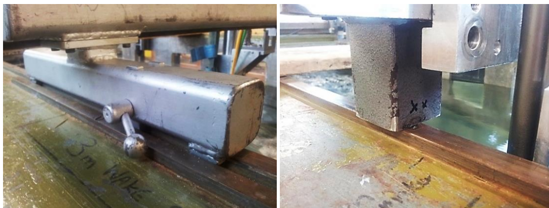
Fig 54: Pre-existing ADV traverse attachment clamp (left), and free-standing foot (right)
