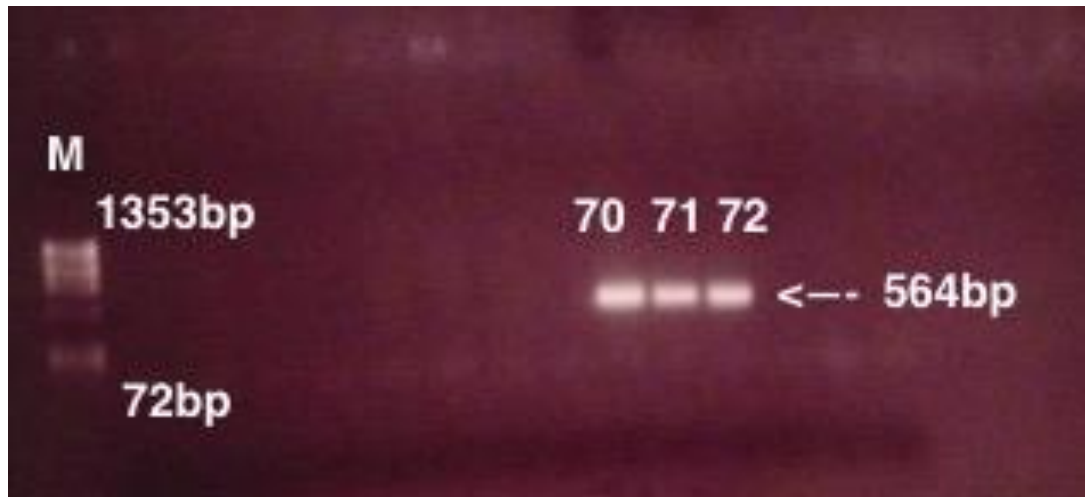
Figure 4.13 Simplex PCR assay using primers to detect bla OXA gene performed on isolates from isolates from the VDL, Leahurst. Isolates 70, 71, 72 appear to show strong amplification of bla OXA-1 . The DNA loading dye DNA/BsuRI (HaeIII) Marker 9, 50 mg (0.5 µg/µl)(ThermoScientific Molecular Biology), was placed on each gel run.
