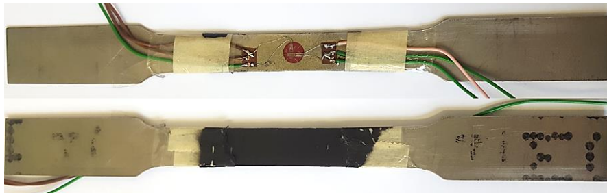
Fig 3.7: Titanium tensile specimen showing the strain gauge rosette which was bonded on one side and black paint on the other side for TSA experiment
