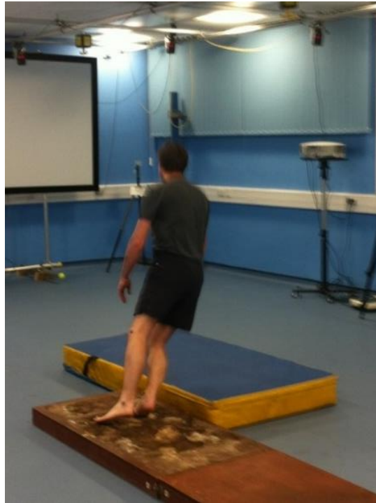
Figure 5.1 Kinematic data collection. The subject falling sideways on to the crash mat. It is possible to see one of the kinematic markers located on the subject's lateral malleolus. This marker corresponds to a green dot on the left-hand side figure.
