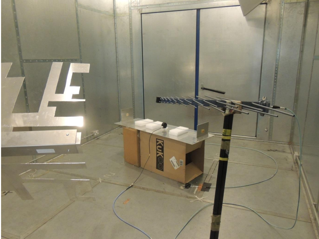
Fig. 7-4. Experiment setup of the random multipath field-to-wire coupling.
