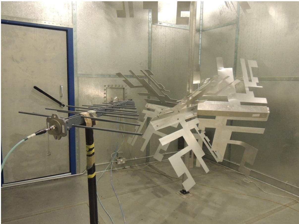
Fig. 7-5. Setup of the transmitting log-periodic antenna.
