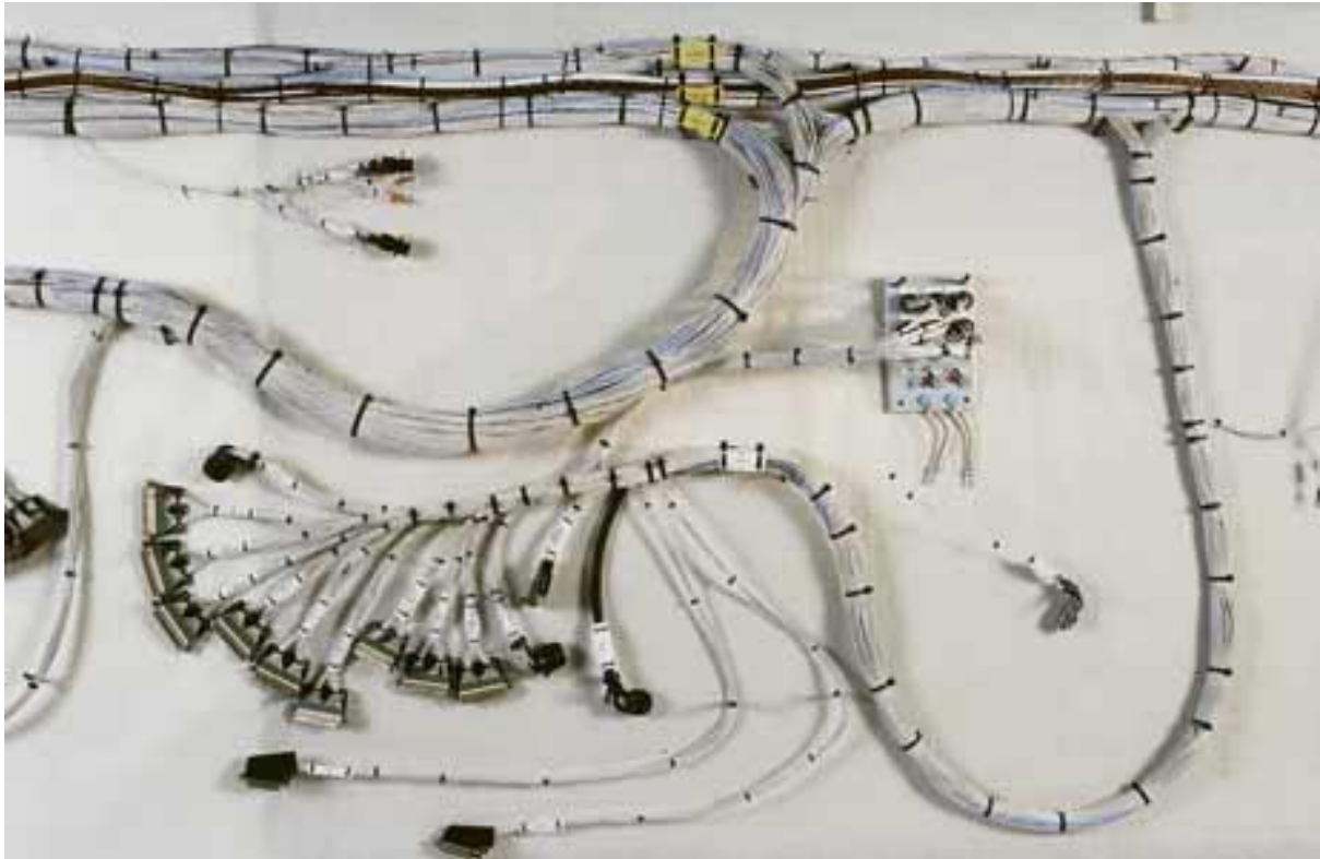
Fig. 1-3. Example of aircraft wiring interconnection [10].
