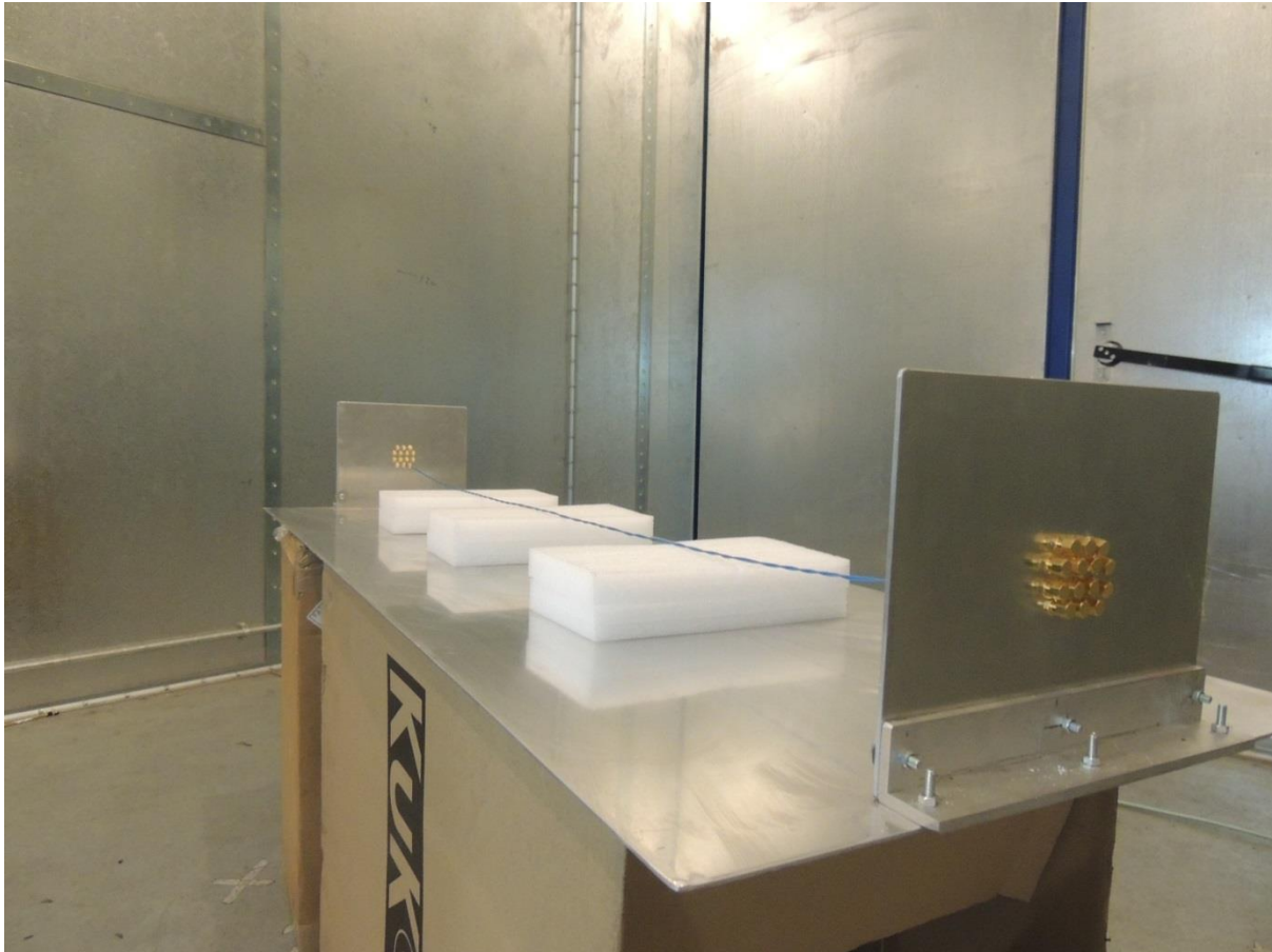
Fig. 7-3. Cable interconnecting system as the DUT.
