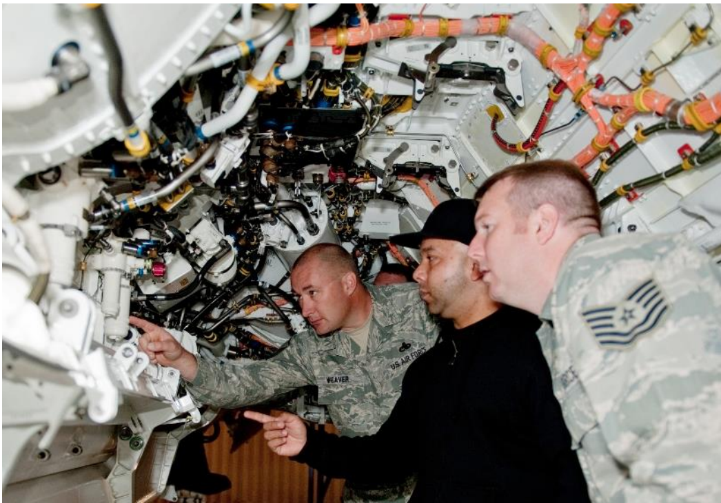
Fig. 1-7. Example of a complex working environment for cable installation in the F-35 JSF military aircraft [22].
