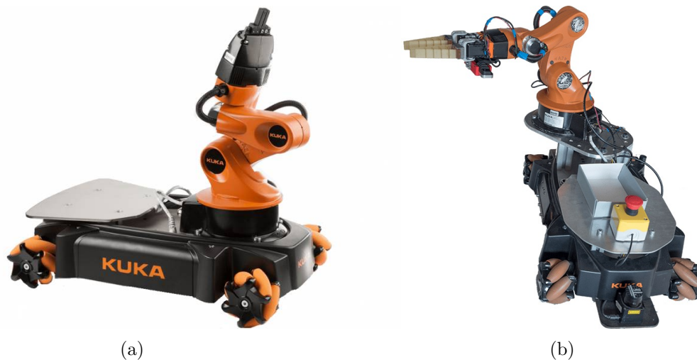
FIGURE A.1: (a) A stock youBot. (b) smARTLab modified youBot.
