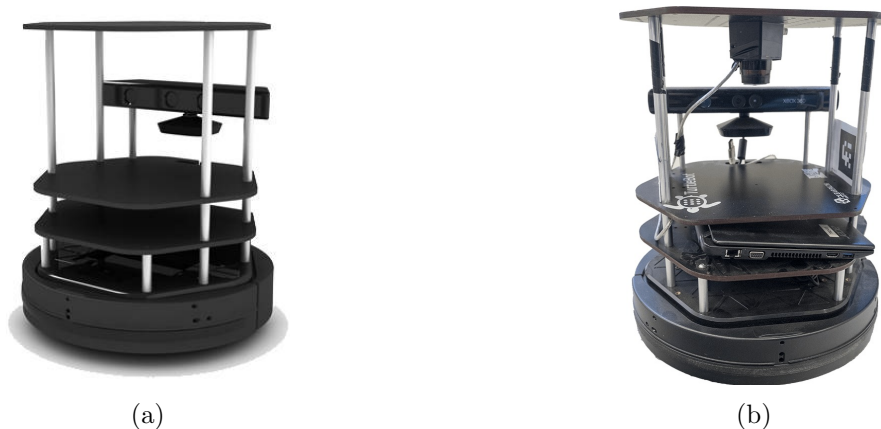
FIGURE A.4: (a) CAD model of a stock Turtlebot. (b) smARTLab modified Turtlebot.
