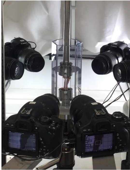
Figure 3. Photograph of the custom-made rig for tensile testing of ligaments.
