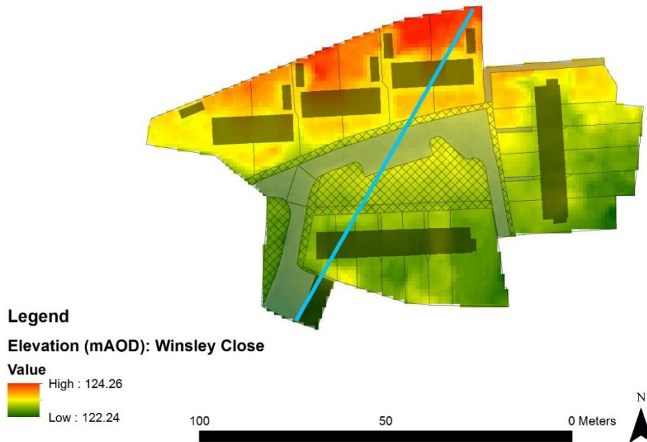
Figure A4.1: Elevation profiles and extracted drainage pathways in Arley Close and Winsley Close.
