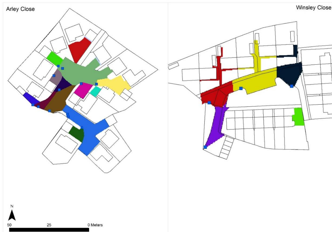
Figure 4.8: Gully drainage areas digitised within Arley Close and Winsley Close. Note that the polygon colours are for illustrative purposes only to differentiate between the different gully areas.
