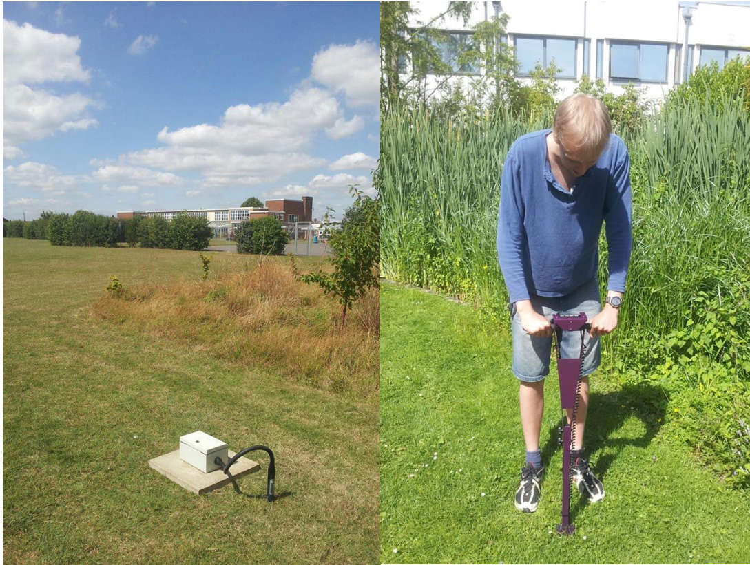
Figure 3.9: Soil moisture monitoring. left) the installed PR2 probe at Swindon Academy (close to Winsley Close), right) field trials with the TDR300 probe.
