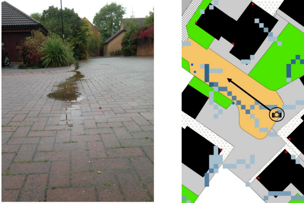
Figure 4.7: Photographic verification (left) of flow accumulation tool output (right) in Arley Close. Camera symbol in (right) shows the location and direction in which photograph is taken. Contains OS data © Crown copyright and database right 2017
