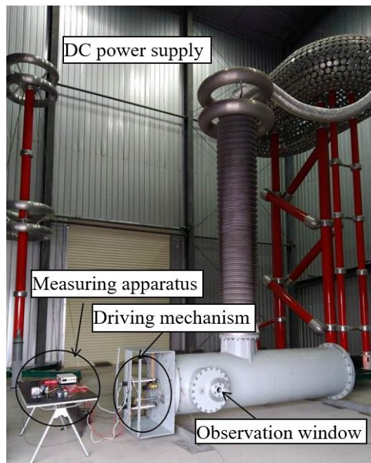
Figure 6-1 A photograph of the experimental system, including DC power supply, test chamber, insulator driving mechanism and potential measuring circuit.
