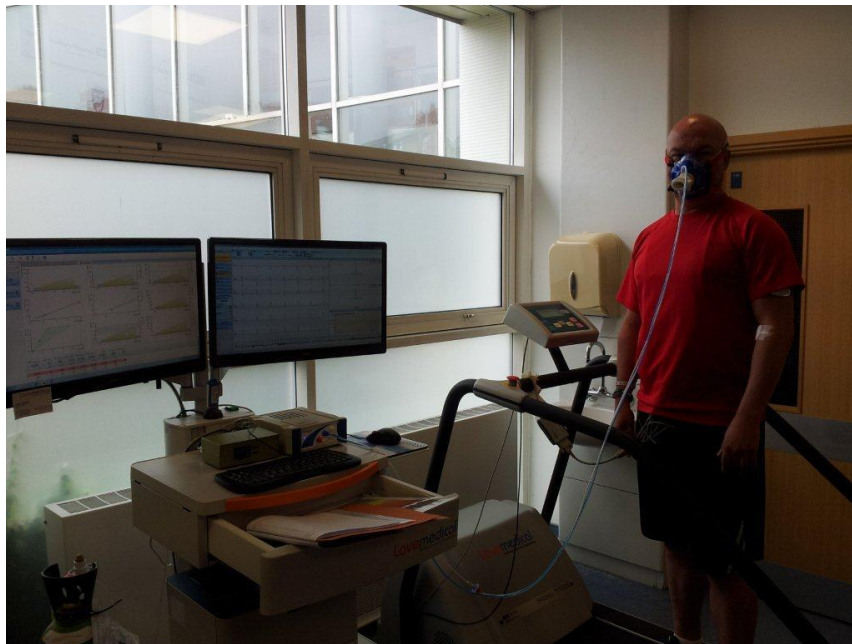
Figure 2.6 A participant set up for assessment of cardiorespiratory fitness (peak oxygen consumption, \dot{V}O_2 peak).
