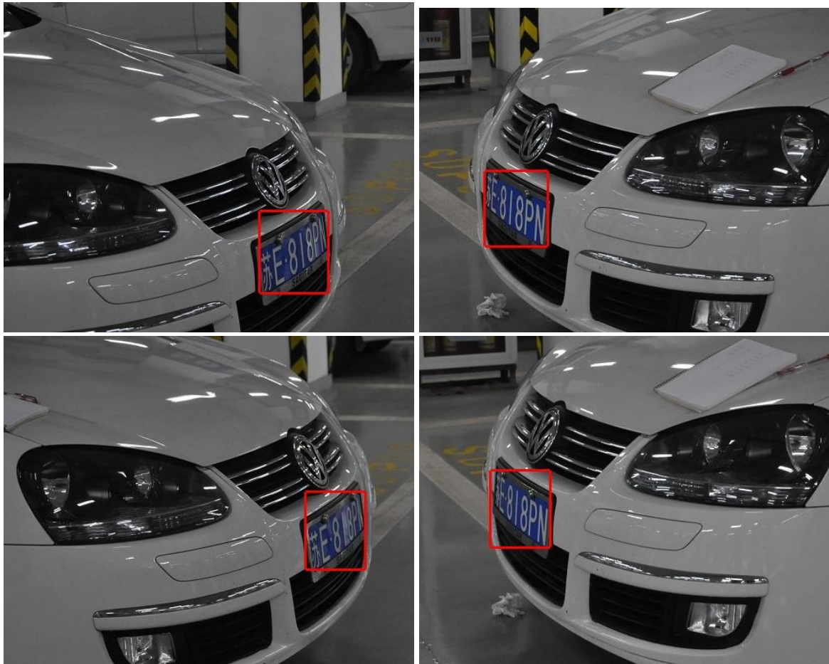
Fig. 7.9 Examples of the skew and tilt dataset. Top: skew degree \pm 70^\circ , bottom: skew degree \pm 75^\circ .
