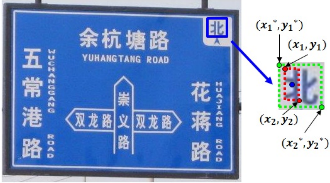
Fig. 8.4 The bounding box regressor adjusts the original bounding box (red) to a updated bounding box (green). The blue point is the central point of original bounding box, and the coordinate encoding scheme uses it as reference point.
