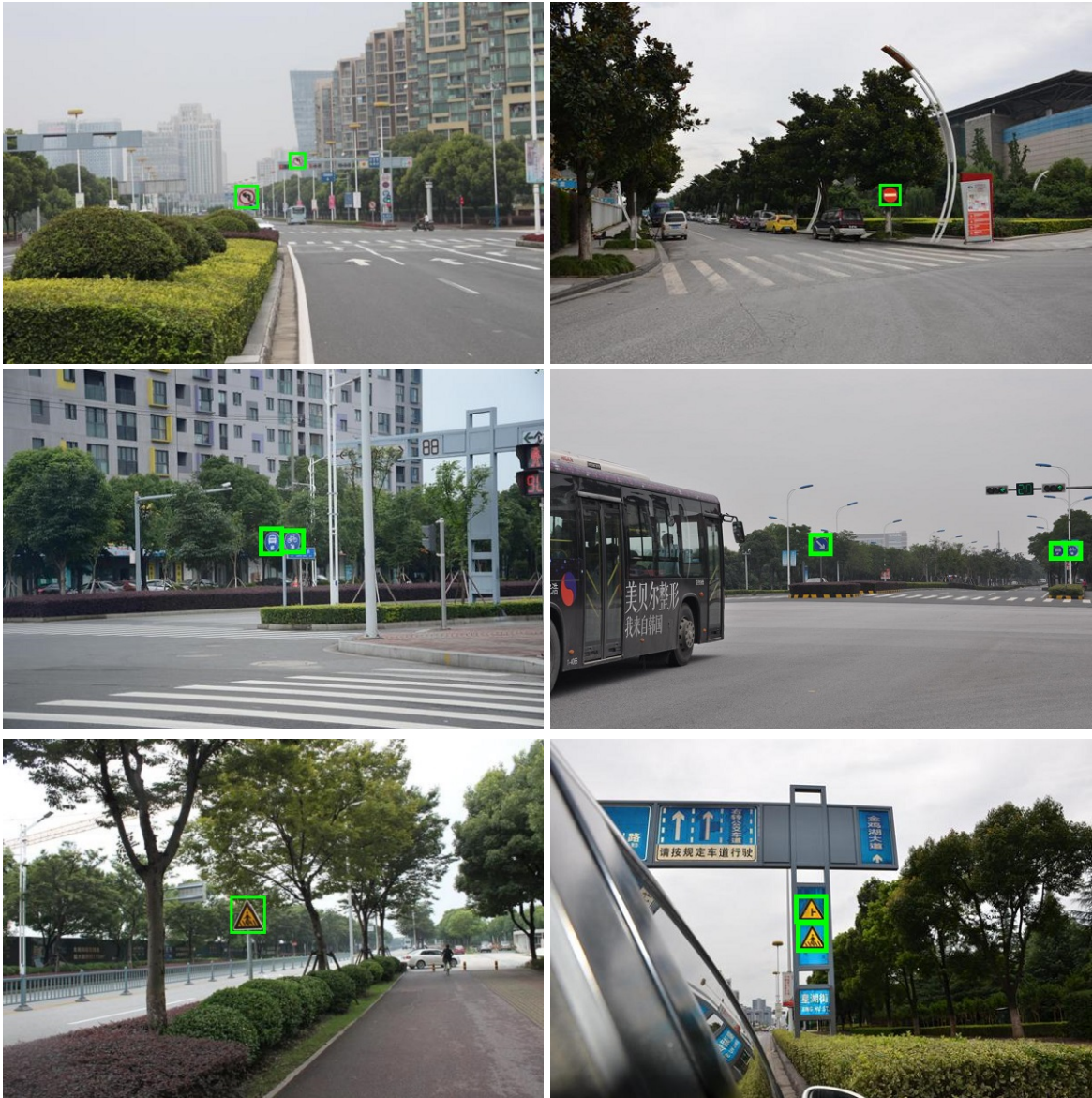
Fig. 3.6 Illustration of example images from the collected data, traffic signs are highlighted with green rectangles. Top: prohibitory signs, middle: mandatory signs, bottom: danger signs.
