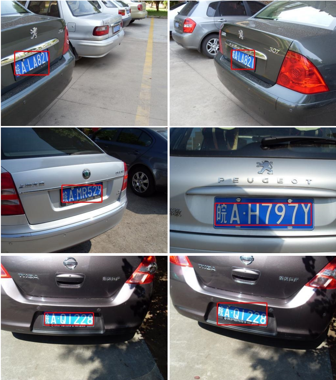
Fig. 7.7 Examples of the LP dataset. Top: skew license plates, middle: weak shadow license plates, bottom: strong shadow license plates.
