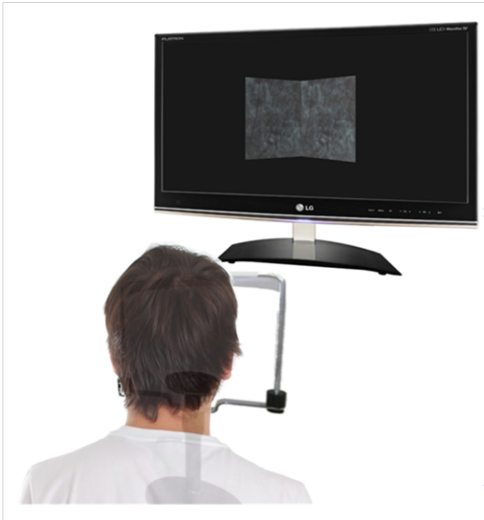
Figure 4-6. Observer's head position when responding to the experiment. Note that the observer responds while still positioned on the chin rest.
