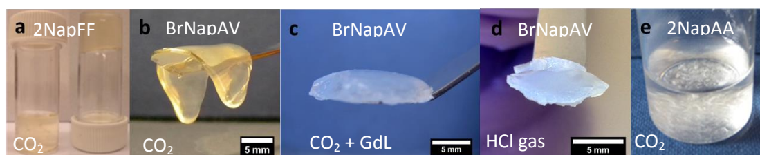
Figure 2.4 – Different behaviours in hydrogel formation when a different gelator or a different self-assembly process are used (a, b and e show data for structurally similar gelators but with different pK_a ) or a different self-assembly process (b, c and d) is used in aqueous solution. Gelators shown here are: (a) 2NapFF ( pK_a 6.0); (b, c and d) BrNapAV ( pK_a 5.8); and (e) 2NapAA ( pK_a 5.1). Solutions (a), (b), (c) and (e) were triggered from high pH with the CO_2 method (Fig. 2.3c) at 1.25 atm for 2 hours. Additionally, BrNapAV sample (c) passed an additional step in the self-assembly process as 16 mg of glucono- \delta -lactone was added to the sample to attain pH 4 (Fig. 2.3d). In sample (d) the BrNapAV hydrogel at 0.5 wt%, pH_f = 2.2 was formed using an HCl gas phase method for 3 hours (Fig. 2.3a).
