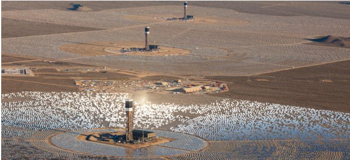
Fig 1.2 The Ivanpah CSP plant in California, producing 390MW of energy
