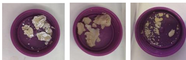
Fig 4.8 Photographs documenting macroscale appearance of PUMCs (left), PUNCs made with 5 %wt surfactants (centre) and PUNCs made with 1 %wt surfactants (right)
