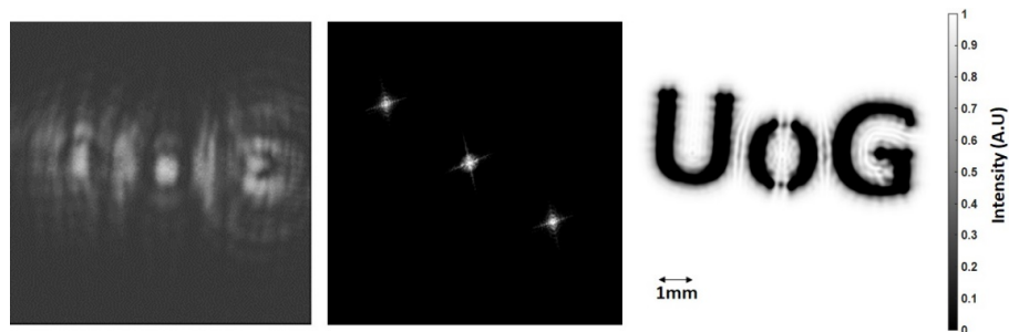
Fig. 3. Simulated interferogram (left), frequency spectrum (mid) and amplitude reconstruction of sample (right).
