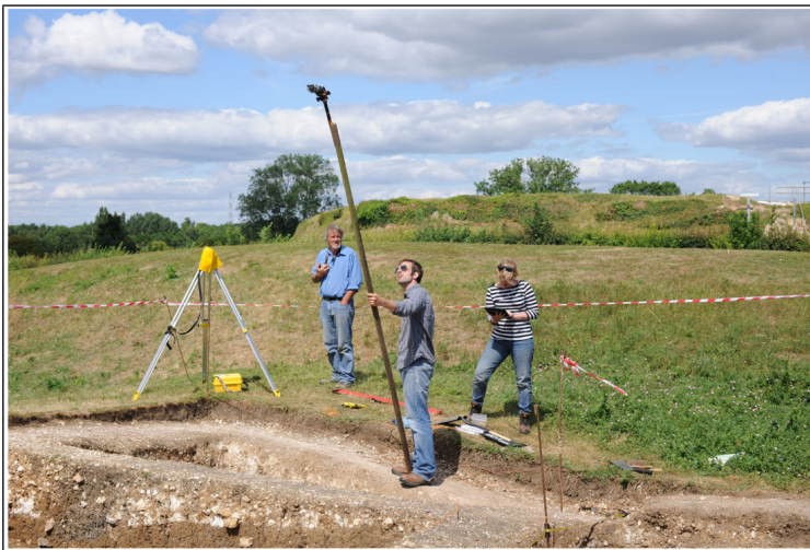
Figure 4.1: Basing House CAT project team members use a GoPro camera, along with the remote controlling iPad app, to photograph the trenches at the end of the excavation season. The images were used to create a photogrammetric model of the excavation
