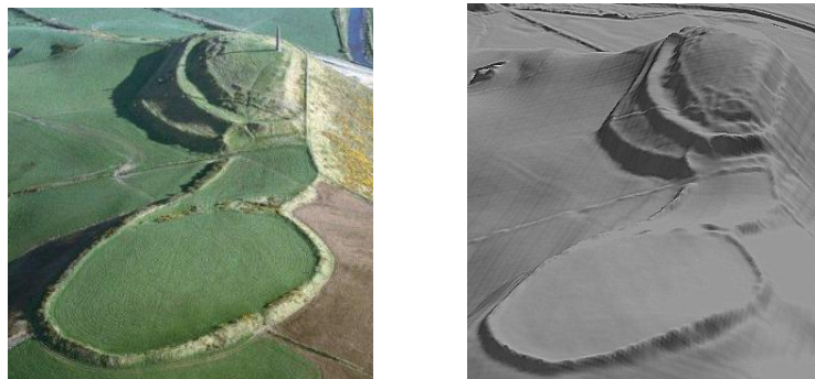
Fig. 1. The two images above show an aerial photograph (left) and a virtual 3D model created with LiDAR data.
