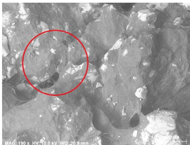
Figure 2. BSE SEM micrograph showing extensive cracking between calcite crystals of the marble at 60x magnification.
