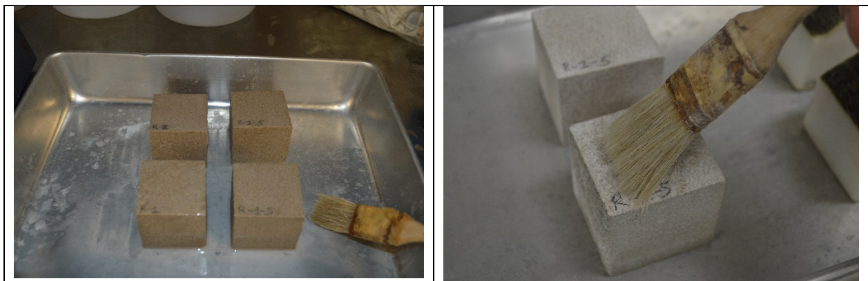
Figure 4. Nanolime I25 brush application to the limestone.
