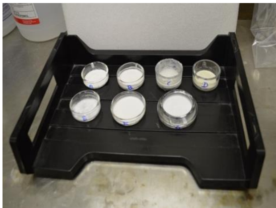
Figure 54. Nanolime samples A-G in the fume hood cupboard at room conditions.
