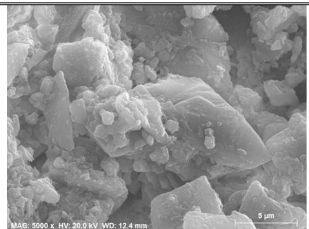
Figure 14. Treated marble at room condition and sprayed with carbonated water [R-2-S]. Left, near the treated surface. Mostly calcite crystals are seen with some framboidal vaterite. Right, an area further down showing apparently new calcite crystals but there are fewer of them (photomicrographs T.F. Lam).
