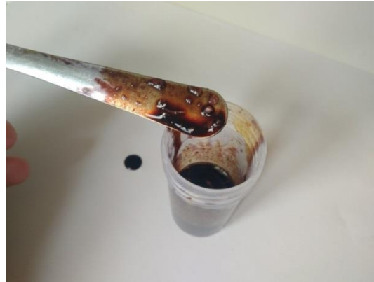
Figure 102. A red-brown color can be seen after the Iodine-KI reagent test due to the presence of amylopectin.
