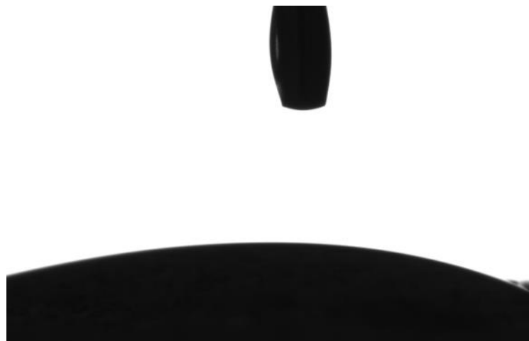
Figure 105. Analysis of the contact angle of sticky rice and substrate
