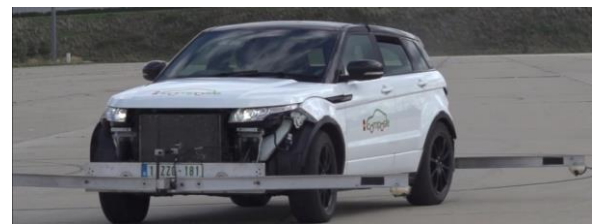
Fig. 4. The iCOMPOSE electric vehicle demonstrator with the Corrsys Datron sensor installed on the front end.
