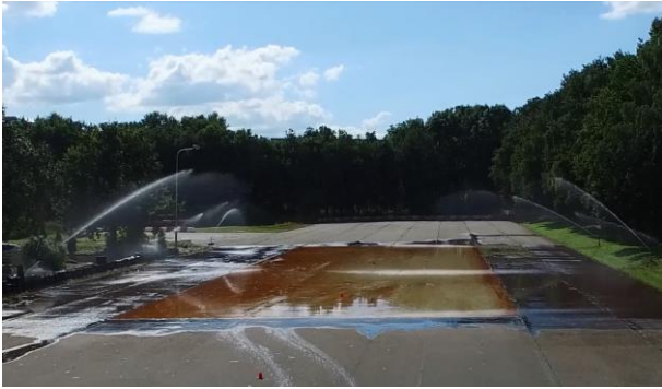
Fig. 5. The Weert proving ground (the Netherlands), with the central low friction area and sprinklers on each side.
