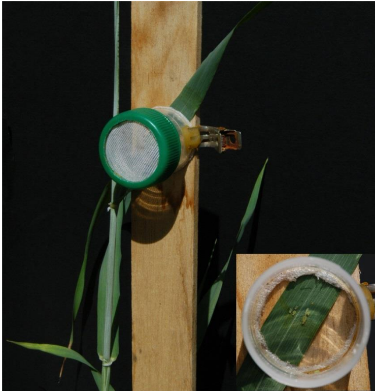
Figure 3.4 Clip cages used to isolate single aphids to determine numbers of nymphs produced.
