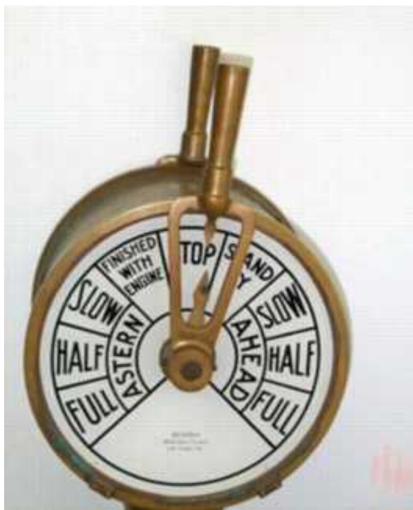
Figure 2.2: A ship's telegraph
